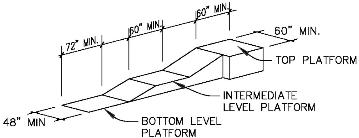
**1010.2 Slope.** Ramps used as part of a *means of egress* shall have a running slope not steeper than one unit vertical in 12 units horizontal (8-percent slope). The slope of other pedestrian *ramps* shall not be steeper than one unit vertical in eight units horizontal (12.5-percent slope).
